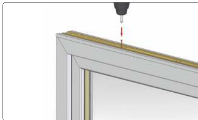
4. Screw the mounted part of the adapter in a distance of 10 cm from the edge. If necessary, drill the hole with a 3 mm drill bit, and then mill with a drill bit of 8 mm.
