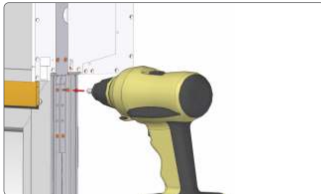
10. Screw the previously prepared steel side connectors to the marked holes with the screws provided.
