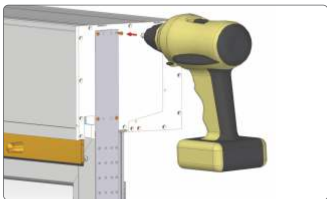
11. Screw the steel side connectors into prepared holes.
