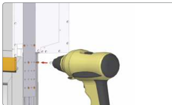
10. Screw the previously prepared steel side connectors to the marked holes with the screws provided.
