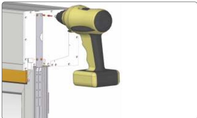
10. Screw the previously prepared steel side connectors to the marked holes with the screws provided.
